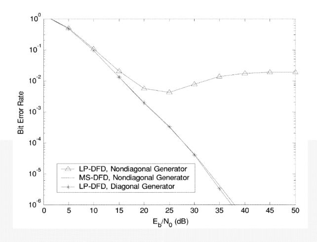
BPSK 3 Tx antennas design with  $f_DT_B=0.03, V=3, N=1$
