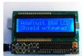
LCD Shield Kit w/ 16x2 Character Display - Only 2 pins used!
