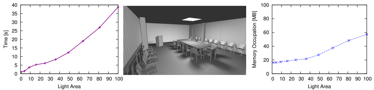
Figure 2.20: Increasing the light size. Left: The time consumption. Right: The maximum memory load reached during the computations. Center: A picture from our tests with the largest area light source (100 times larger than the smallest one. This corresponds to a square whose side is exactly the width of the conference table).
